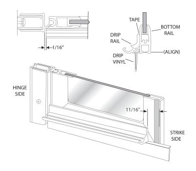
Adjust the drip vinyl [N] by sliding it left or right until it just touches the curb. Trim the vinyl (flush with the hinge end a nd notch 1/4" longer than the drip rail as shown on the strike end). Secure it with one #6 x 3/8" truss head screw [S] in the hinge end of the drip rail.
