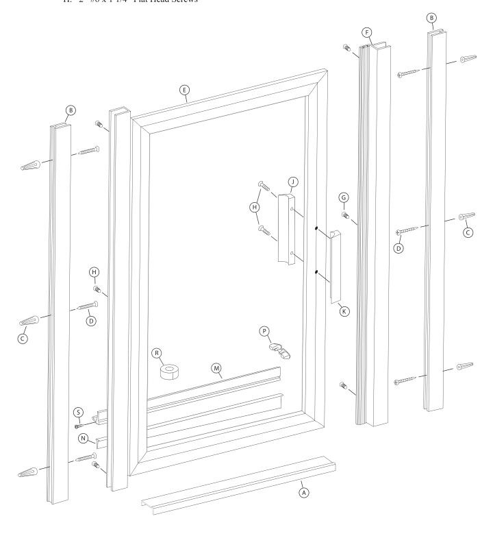
The Continuous-Hinge Door is completely reversible and may be installed hinge-left or hinge-right. Refer to the illustration to determine the correct position for your installation. For maximum waterproofing, the hinge jamb should always be opposite the shower head. These instructions depict a hingeleft installation.
