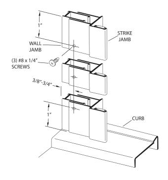
Slide the door panel [E] over the other wall jamb [B] until the door panel and the strike jamb [F] can meet. With the door closed and the latch magnets engaged, the proper door panel to strike jamb clearance is 1/8" (see illustration). Mark the hinge jamb's location on the wall jamb with a pencil.
