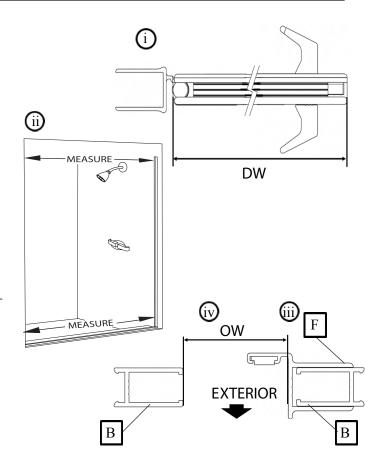
Inside the shower enclosure, drill two 1/8" holes through the strike jamb [F] and into the wall jamb [B] 3/8" to 3/4" from the wall and approximately 1" vertically from each end of the strike jamb. Drill a third hole centered between the first two, then enlarge the three outer holes with a 3/16" drill for clearance on the self-tapping screws. Attach the strike jamb permanently with three #8 x 1/4" truss head screws [G].
