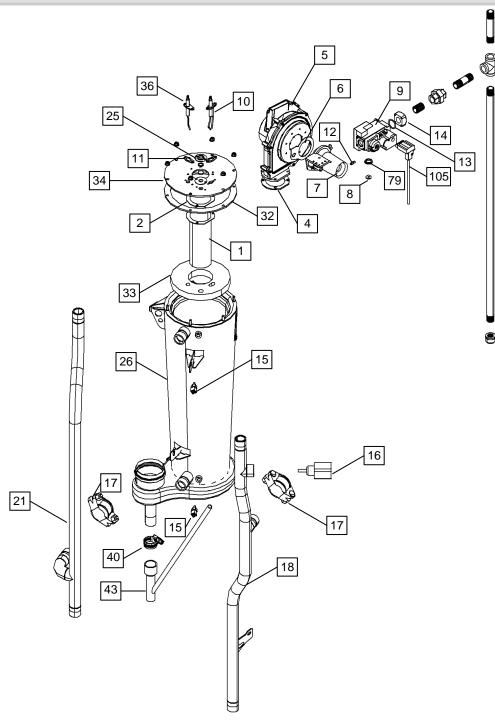
Figure 17-1(a) Tft60-110 Heat Engine and Gas Train
