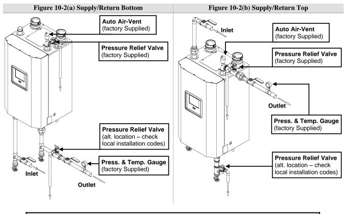
Boiler Outlet and Inlet water connection location varies between models; reference the applicable figure for correct location.
