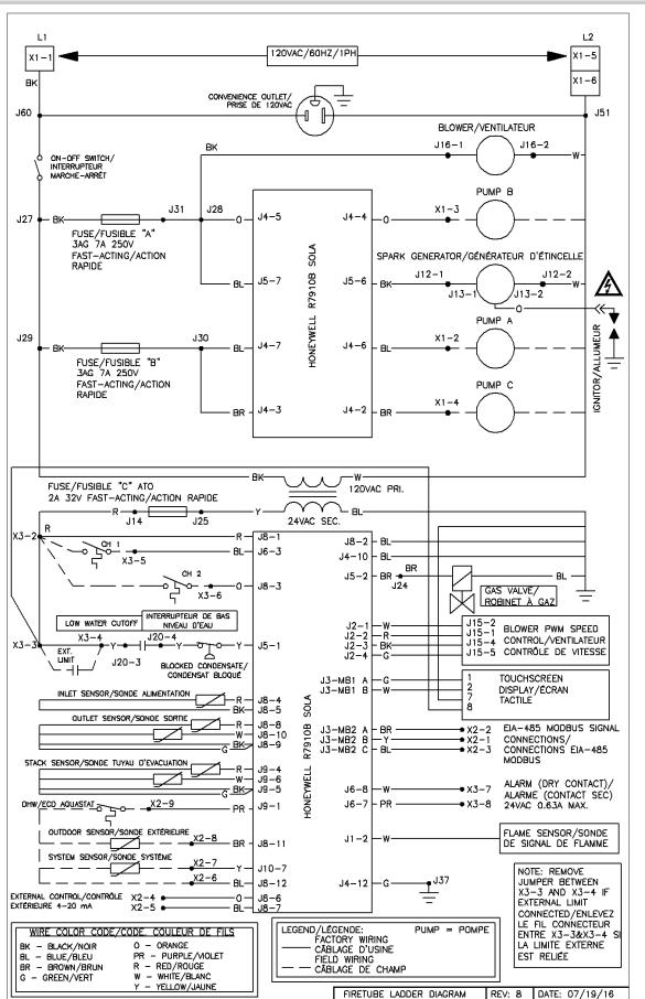
Figure 13-2 Tft Ladder/Logic Diagram
