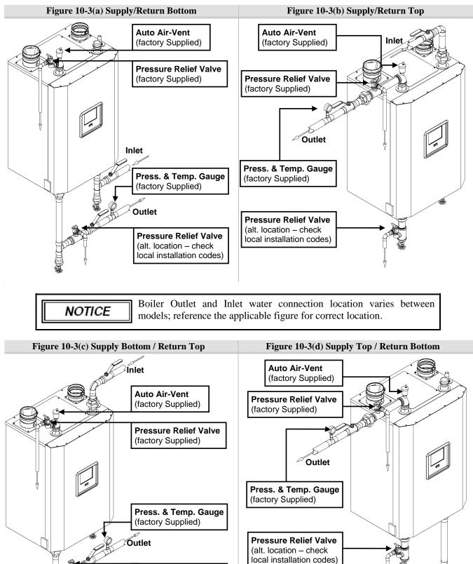
Pressure Relief Valve (alt. location – check local installation codes)
