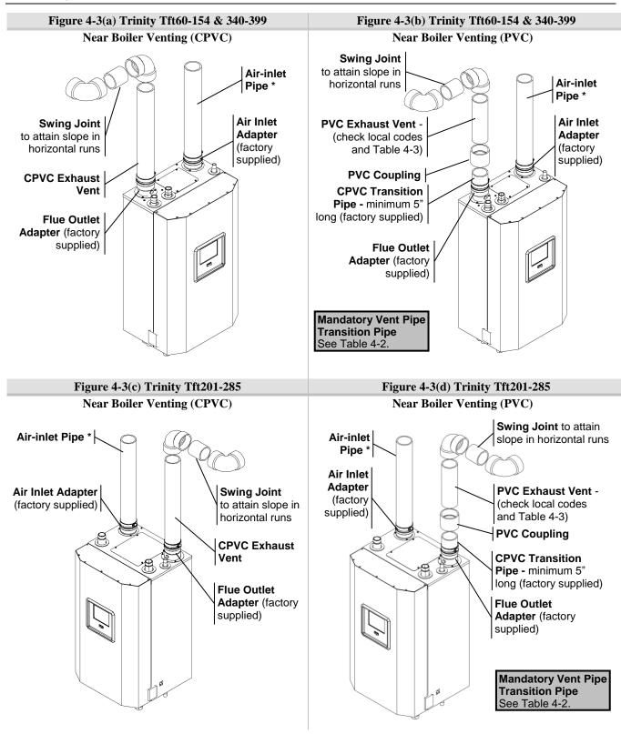
\* Air-inlet - check with applicable local codes for acceptable pipe material.
