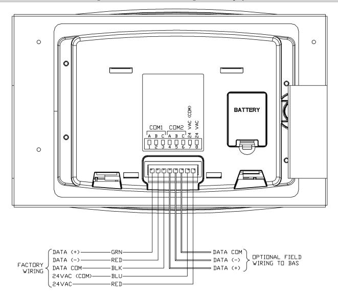
Figure 12-3 COM2 Modbus Wiring (Rear of Display)
