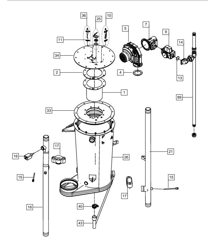
Figure 17-1(c) Tft285-399 Heat Engine and Gas Train (Tft340-399 Illustrated)
