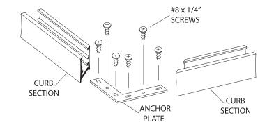
The curb should sit near the centerline of the sill. If required, use a file to round the lower ends of the curb assembly to fit the shower sill properly.
