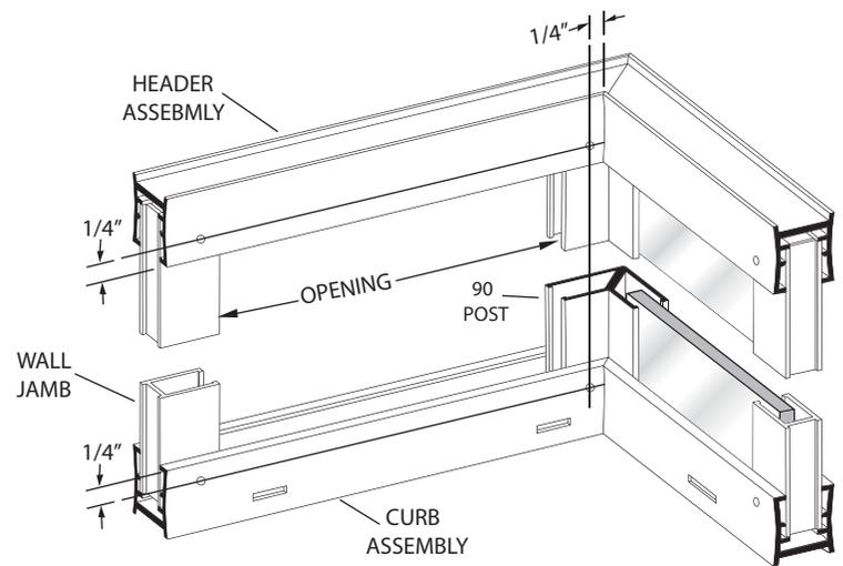
**CAUTION:** Slide the glass panel away from the wall jamb before drilling to prevent breakage.
