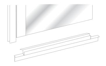
Align the deflector [CC] to the bottom of the door with the hinge side notch over lapping the hinge, then mark the strike side even with the door edge cut deflector at that point.
