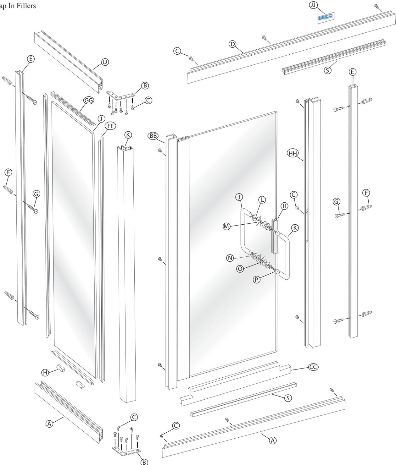
**1** The BASCO 1414/1714 Infinity Shower Door Panel is completely reversible and may be installed hinge-right or hinge-left. The door may hinge from the wall or from the center-post. Using the illustration, determine the correct position for the door in your particular Infinity installation. This instruction sheet depicts a hinge-right installation.
