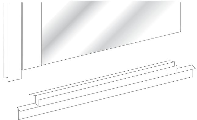
**14** Align the deflector [CC] to the bottom of the door with the hinge side notch over lapping the hinge, then mark the strike side even with the door edge cut deflector at that point.
