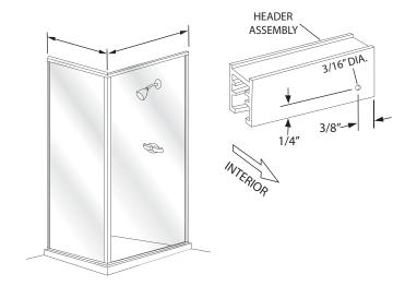
Press the header assembly [D] over the wall jambs [E] and the 90° post [K]. Check the post for plumb. Adjust as required by varying the overlap of the header over the wall jambs. In some cases, you may need to trim the ends of the header where it meets the wall. The minimum horizontal dimension for the door opening is the door panel width (see the graphic in Step #9) plus 1/2", maximum is the door panel width plus 1 3/4".
