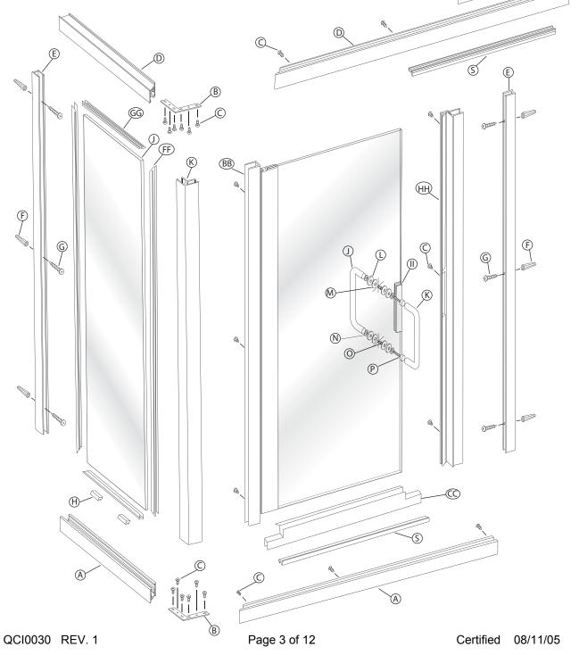
The BASCO 1414/1714 Infinity Shower Door Panel is completely reversible and may be installed hinge-right or hinge-left. The door may hinge from the wall or from the center-post. Using the illustration, determine the correct position for the door in your particular Infinity installation. This instruction sheet depicts a hinge-right installation.
