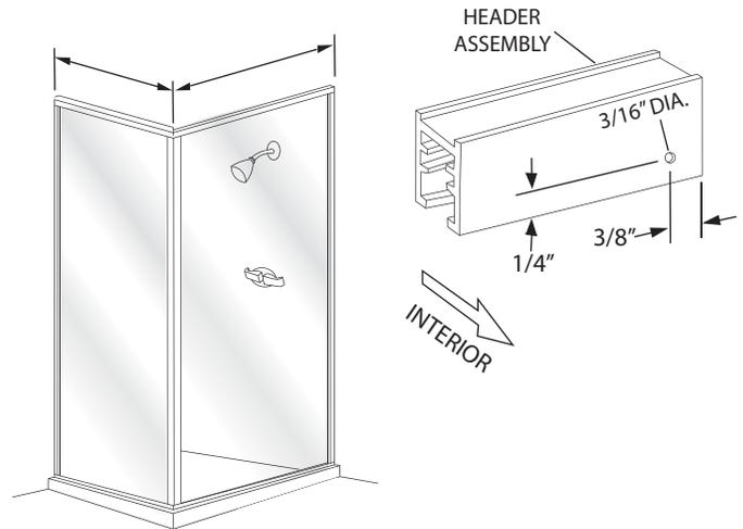
**8** Press the header assembly [D] over the wall jambs [E] and the 90° post [K]. Check the post for plumb. Adjust as required by varying the overlap of the header over the wall jambs. In some cases, you may need to trim the ends of the header where it meets the wall. The minimum horizontal dimension for the door opening is the door panel width (see the graphic in Step #9) plus 1/2", maximum is the door panel width plus 1 3/4".
