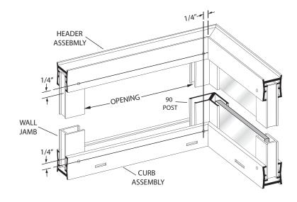
Orient the door to the opening (either hinge right or hinge left). Place the door in the opening with the door hinge over the wall jamb or post.
