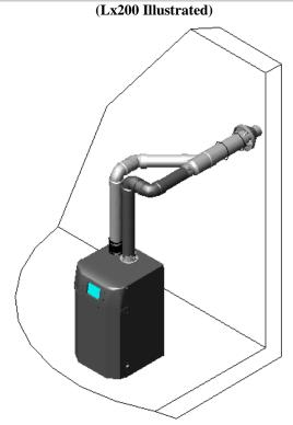
Figure 4-6(b) Two-Pipe Sidewall Termination (Lx200 Illustrated)
