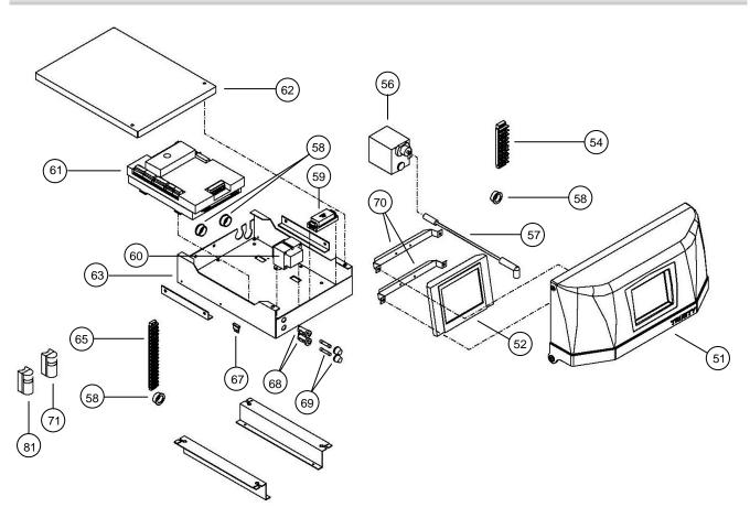
Figure 16-4 Cabinet, Vent and Air-Intake Parts (Lx300-400)
