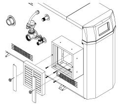
2 Secure filter kit using factory screws removed in step 1. Reuse the factory gasket.
