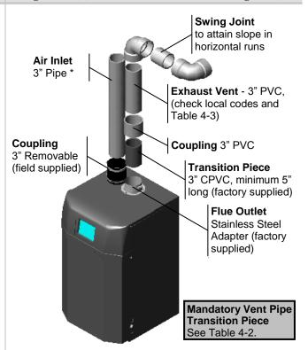
Figure 4-3(a) Lx300-400 Near Boiler Venting (CPVC)
