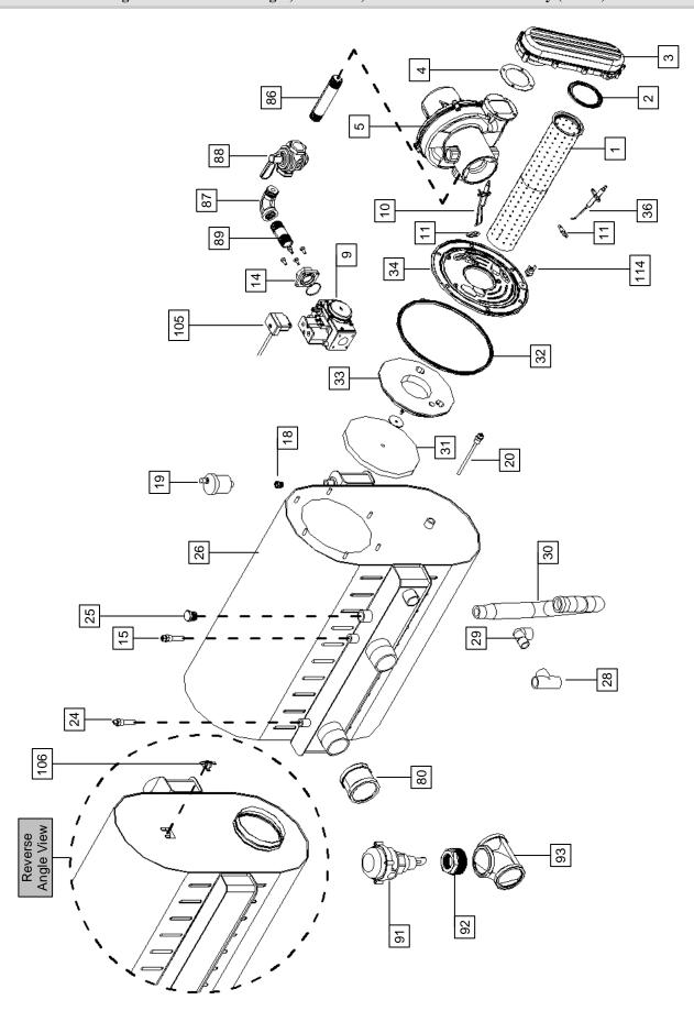
Figure 16-8 Heat Exchanger, Gas Valve, Blower and Burner Assembly (Lx600-800)
