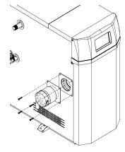
• Remove factory appliance air-inlet adapter; keep screws from installation of filter kit
