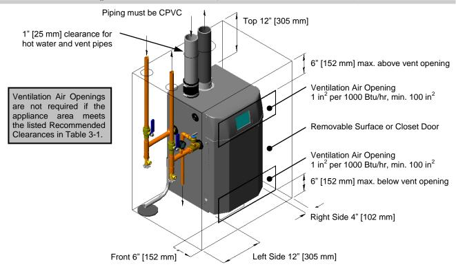
Figure 3-1(b) Closet Installation, Minimum Clearances (Lx300-400)
