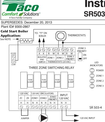
**Operation:** When any thermostat calls for heat, the appropriate circulator is energized and the isolated end switch (X and X) will start the boiler.
