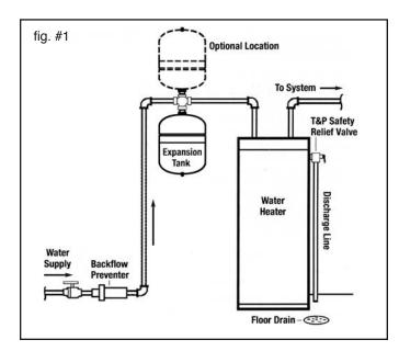
Before turning on the water supply to the system, open a hot water faucet to prevent any damage to the water heater and remove air from the system piping. Turn on the water supply and inspect the installation for water leaks paying close attention to the connection between the expansion tank and the piping.
