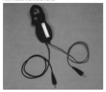
The Amprobe is a multi-range, combination ammeter and voltmeter.
