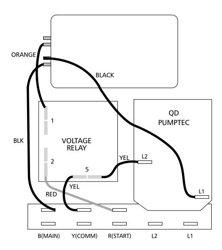
CENTRIPRO CONTROL BOX WITH PUMPTEC INSTALLED
