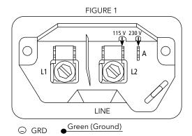
Align black plug to 115 V or 230 V arrow. ½ HP wired 115 V, ¾ HP and up wired 230 V at factory.
