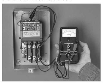
Open master breaker and disconnect all leads from starter to avoid damage to meter or electric shock hazard. Connect the ohmmeter leads as shown above.
