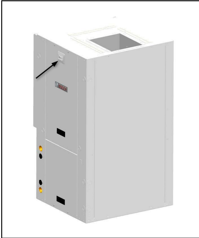
Fig. 69 Vertical (VT) Unit WIM Mounting Location
