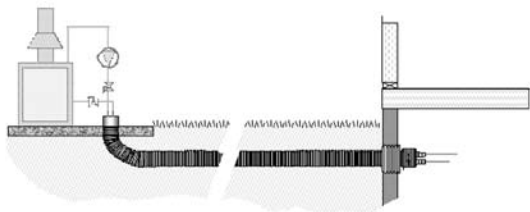
Figure 3-2: Reduce Below-grade Connections
