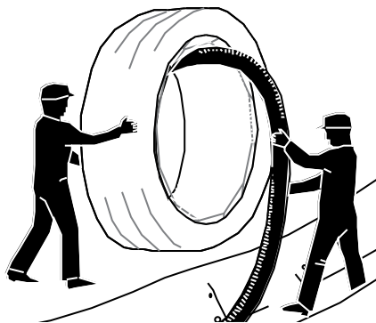
Figure 4-3: Uncoiling Short Lengths
