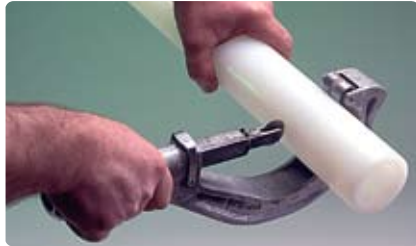
Figure 4-24: Cut the Pipe
