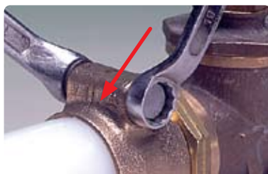
Figure 4-32: Tighten the Fitting
