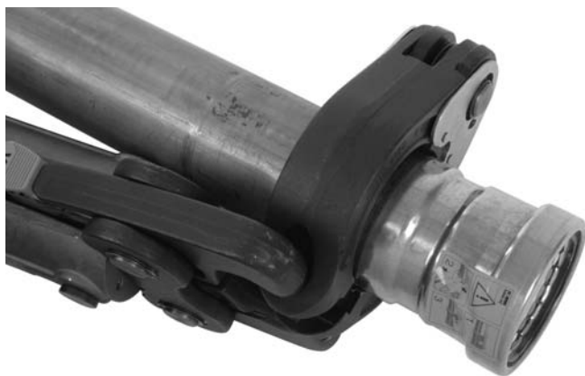
Figure 14C – Placing V2 Actuator Into XL-C Ring Pockets At An Angle For Additional Clearance
