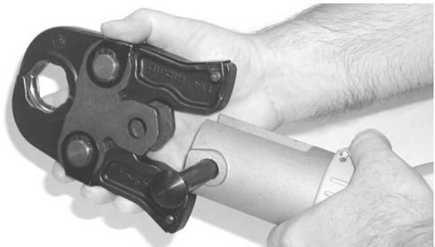
Figure 6 – Pulling The Jaw Set Mounting Pin Out
