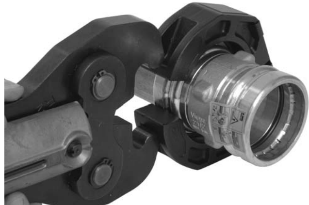
Figure 14A – Placing R2 Actuator Tips Into XL Ring Pockets
