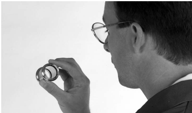
Figure 7A – Inspection of the ProPress Fitting per the Manufacturer's Instructions
