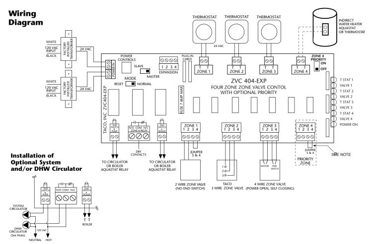
**Operation/External Diagnostics:** When any thermostat calls for heat, the appropriate zone valve is energized and the yellow light goes on. When the zone valve is fully open, the red light goes on and energizes the end switch relays. The green light should always be on, indicating that power is connected.
