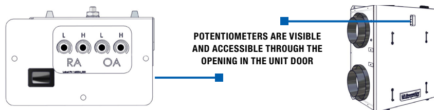
FIGURE 4.6.1 FAN SPEED CONTROL POTENTIOMETERS
