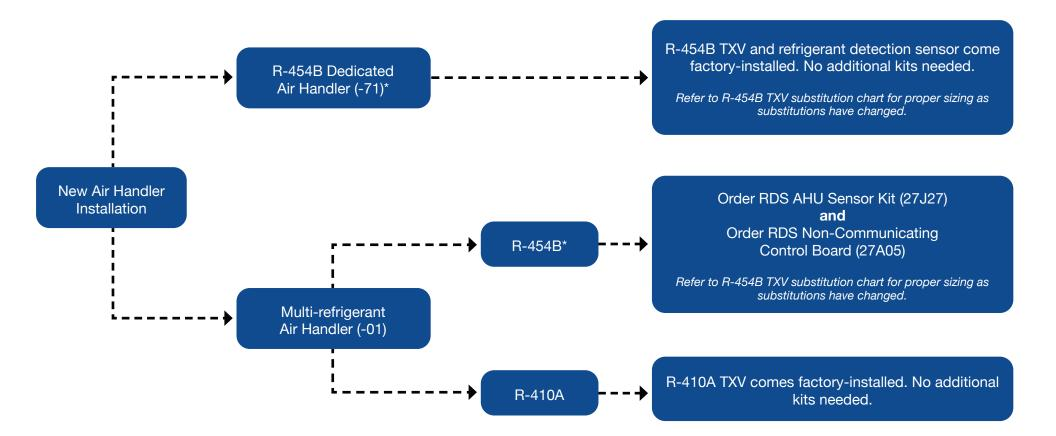
\*For secondary joints, please see the air handler installation instructions for additional requirements. RDS boards and sensors are exclusively for use with Allied Air equipment.
