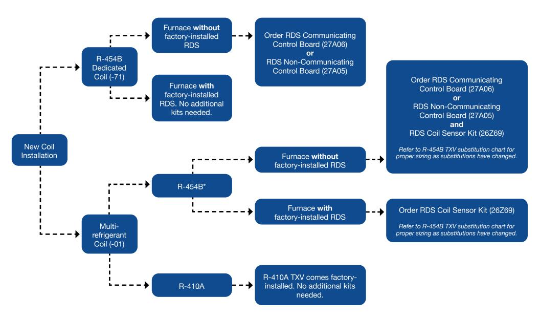
\*For secondary joints, please see the coil installation instructions for additional requirements. RDS boards and sensors are exclusively for use with Allied Air equipment.
