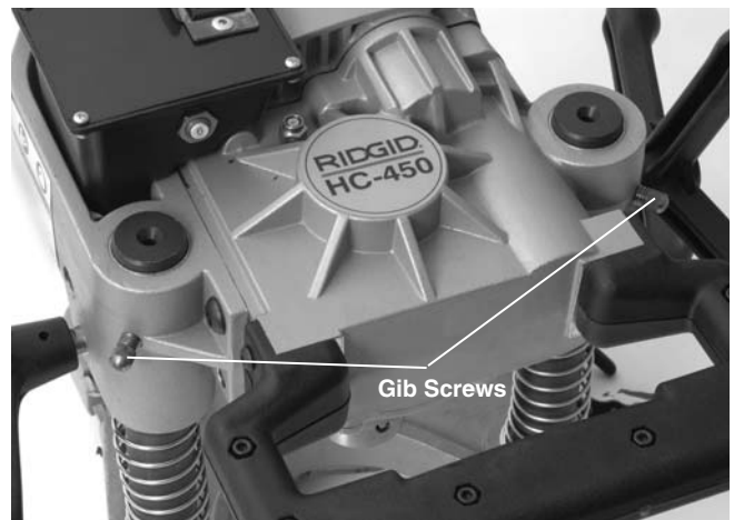
Figure 13 – Adjusting Gib Screws
