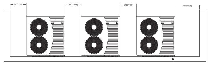
Unit shall be mounted per local codes and high enough off ground to allow for proper condensate drainage and snow clearance.
