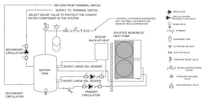
\*Autofill system is suggested but not required by SpacePak. If such installation is desired or required by local code, the Autofill MUST draw from a reservoir of pre-mixed glycol/water solution. Filling directly from a well or municipal water source may introduce contaminants and will dilute the glycol solution in the event of a system leak. This may impact warranty coverage.
