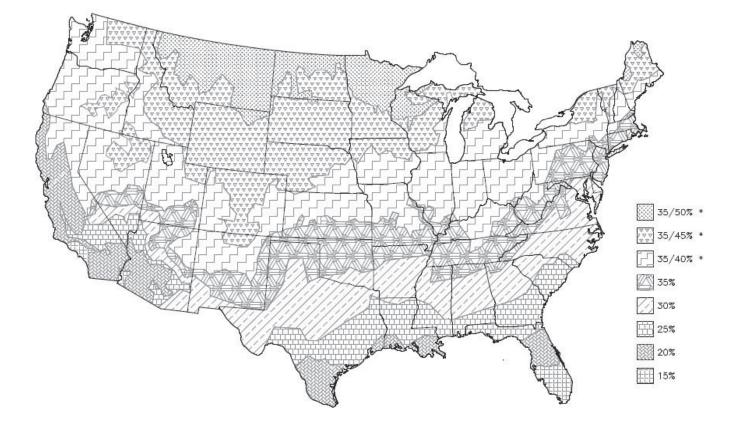
\* A 35% concentration will prevent solid freezing, and protect from bursting, in all conditions. However, this solution will become a thick sludge at extremely low temperatures, possibly resulting in pump overloading, pump damage, or high pressures. Therefore this concentration should only be used in systems that will remain inactive during the winter. Use the higher value shown for systems that must start and run at the coldest temperatures.
