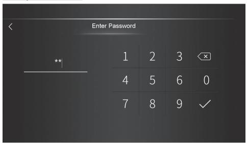
To unlock, simply press the lock key again and enter the code "22" when prompted. Press enter and the screen will be unlocked again.
