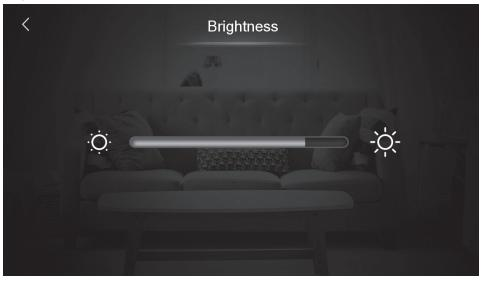
The brightness key allows the user to adjust the screen brightness. Press the brightness bar to the right to make the display brighter and the left on the brightness bar to make the display less bright.
