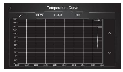
The curve key allows a user to visually see (in real time and historical) the operational curves of the inlet water, outlet water and ambient on graph of temperature versus time period.
