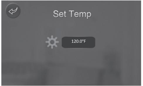
This can be adjusted by pressing the temp (on the screen) which opens a new screen and then entering in a numeric value within specified parameters in the control (see parameter chart for min and max settings). Once a target is set, the user will need to press "enter" to save the set point. This should return the user to the target set screen where they will see the new setpoint has been saved. Press the return key to return to the main interface.
