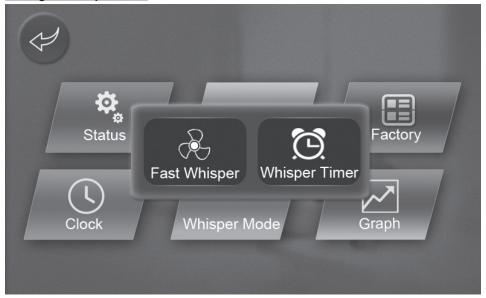
Note: Whisper Mode and Whisper Timer are only visible if enabled by parameter H22.
