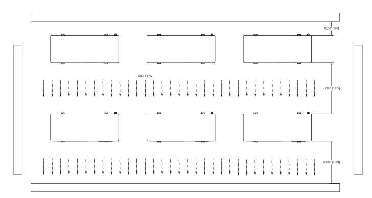
CLEARANCES SHOWN ARE ASSUMING NO WALL EXTENDS MORE THAN 6" ABOVE THE TOP OF THE HEAT PUMPS, THERE IS NO OVERHEAD ROOF, AND THERE ARE NOT MORE THAN TWO BARRIER WALLS ADJACENT TO THE UNITS ALL DIMENSIONS ARE IN INCH"[mm] AND CLEARANCES APPLY TO ALL UNIT SIZES
