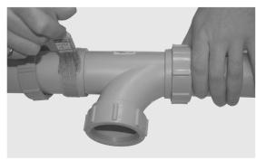
7. Hand-tighten the nut, then tighten using a spanner wrench. For stability and leverage, two spanner wrenches may be used as depicted. The nut must be tightened to achieve full thread engagement.
