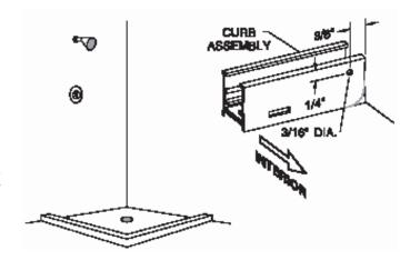
Place the two wall jambs [E] into the ends of the curb assembly [A]. Masking tape may be used to hold the curb in place during this operation. Plumb the jambs and mark the hole locations on the wall. Remove all parts and drill the walls for mounting hardware.
