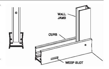
Wipe the shower walls and sill, curb assembly [A] and wall jambs [E] with a clean, dry cloth to remove any dust or debris. Apply a 1/4" bead of caulk along the inside of both of the pencil lines marked in Step #3. Carefully replace the curb in the exact position marked. Caulk the inside of the curb ends where they meet the wall. Caulk generously around the anchor plate [B], screws [C], and the insides of the mitered joint.
