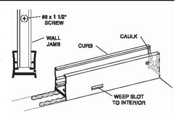
Place the setting blocks [H] in the curb assembly [A] as shown to support the two fixed glass panels [J]. The setting blocks should be positioned approximately 3" from each corner of the glass panel. It should rest on the setting blocks and be engaged approximately 1/2" into the wall jamb [E]. A strip of masking tape 1/2" from each vertical edge of the glass will aid alignment.
