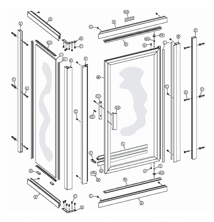
The BASCO 145/745 Thin-Line Shower Enclosure is completely reversible and may be installed pivot-left or pivot-right. The door may pivot from the wall or from the center post. Using the diagram, determine the correct position for the door in your particular Thin-Line installation. This instruction sheet depicts a pivot-right installation.
