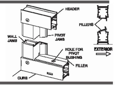
Pull the bottom end of the pivot jamb [N] tight to the curb filler [R] and plumb the jamb. Drill two 1/8" holes thru the pivot jamb and into the wall jamb [E] 3/8" to 3/4" from the wall and approximately 1/4" vertically from the ends of the jamb. Drill a third hole centered between the first two and enlarge the three outer holes with a 3/16" drill for clearance on the self-tapping screws. Attach the pivot jamb permanently with three #8 x 1/4" truss head screws [C].
