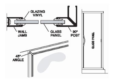
Cut four pieces of the larger vinyl [GG] 1/2" longer than the horizontal opening and trim the ends on a 45° angle. Install the top exterior vinyl starting at both ends and working toward the middle. Be careful not to stretch the vinyl.
