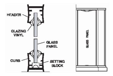
Carefully caulk the interior jamb-to-wall and curb-to-base joints. For appearance, you may wish to caulk the exterior joints as well. We recommend you wait twenty-four hours before the first shower to allow the caulking to cure properly.
