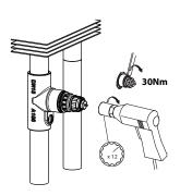
Fasten built-in valve with a torque of 30 Nm +/- 10%. 21M spanner.
