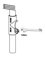
Fasten air-vent with a torque of 10 Nm +/- 10%. 13M spanner.
