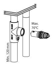
Insert the built-in valve into the steel valve housing
