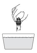
Lubricate valve insert by dipping in water.
