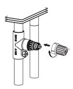
5. Fit protection cap. Tighten cap.
