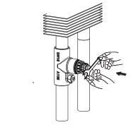
Test operation of valve spindle, by pushing the pin.
