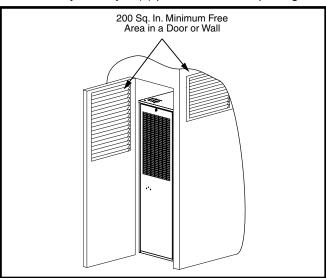
Figure 6. Closet Installation
