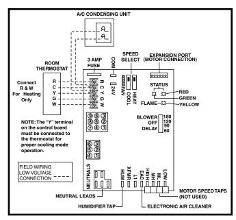
Figure 15. Low Voltage Field, Four-wire Heating/Cooling Applications
