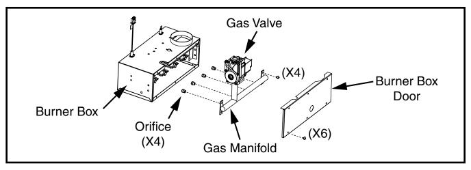
Figure 14. Orifice Removal
