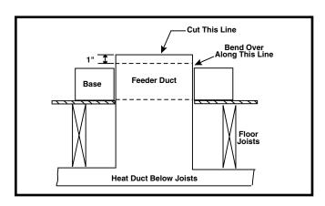
Figure 9. Feeder Duct Installation
