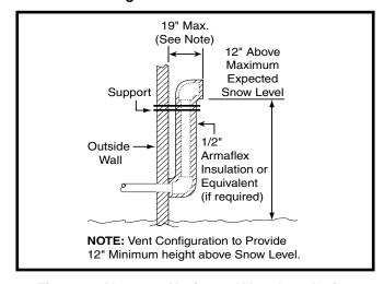
Figure 3. Alternate Horizontal Vent Installation
