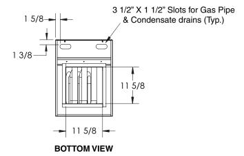
Figure 18. Furnace Dimensions
