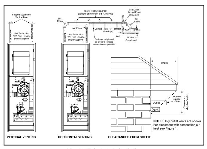
Figure 20. Horizontal & Vertical Venting
