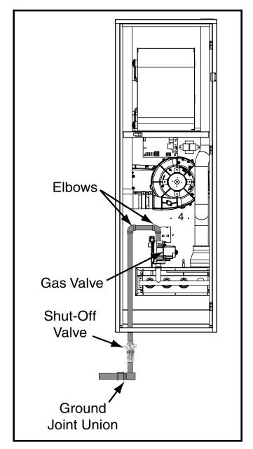
Figure 12. Typical Gas Connections
