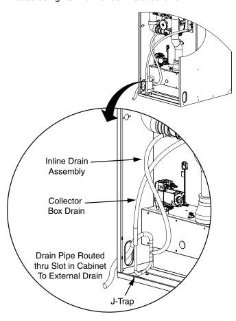
Figure 11. Condensate Drainage
