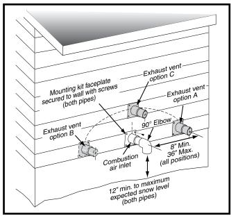
Figure 1. Inlet & Exhaust Pipe Clearances
