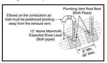
**Figure 4. Vertical Vent Termination**
