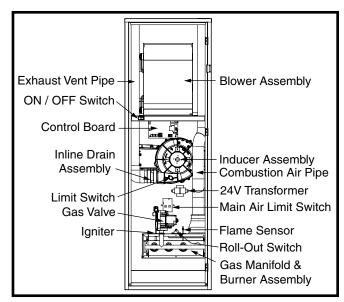
Figure 17. Furnace Components
