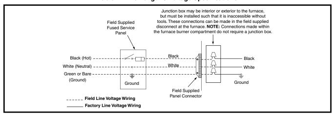
Figure 16. Line Voltage Field Wiring
