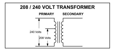
Figure 7. Converting Unit from 240VAC to 208VAC
