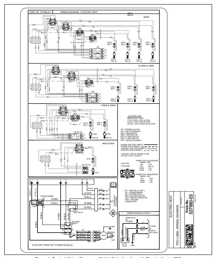
Figure 1. Typical Wiring Diagram – 7AH1AC Air Handler with Electric Heat – PSC
