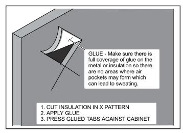
Figure 20. Repairing Insulation
