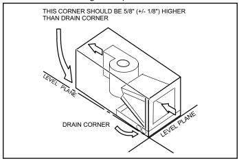
Figure 15. Sloping the Unit for Proper Drainage
