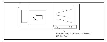
Figure 13 . Left-Hand Discharge Configuration
