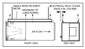
Figure 12. Suspending Horizontal Unit
