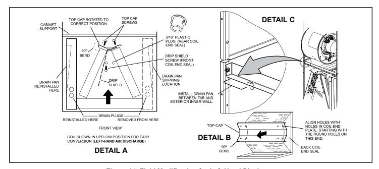
Figure 14. Field Modification for Left-Hand Discharge
