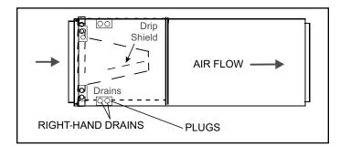
Figure 11. Right-Hand Discharge Configuration
