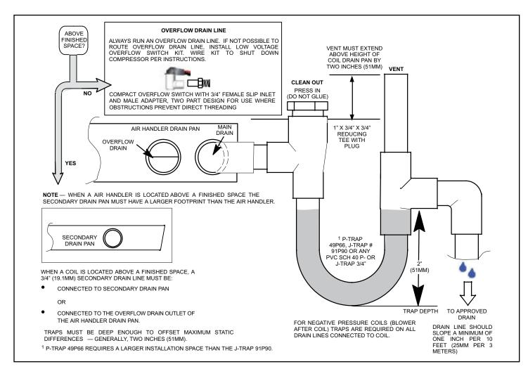
Figure 17. Typical Main and Overflow Drain
