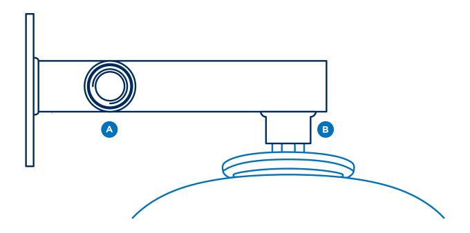
The 4Pro Potable Thermal Expansion Tank Bracket combines many functions, one of which is offering the ability to read the system pressure at any time. When the valve is shut, it is possible to use it to drain the tank or to do its maintenance. Once the tank is drained, it is easy to check that its pressure is equal or higher than the municipal system and adjust it if it is not the case to ensure its proper functionning.
