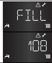
Figure 80 - Shut-Off Error for Low Water Pressure
