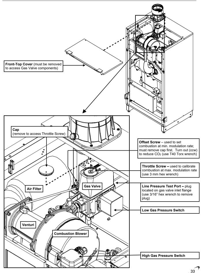
Used to calibrate combustion at max. modulation rate
