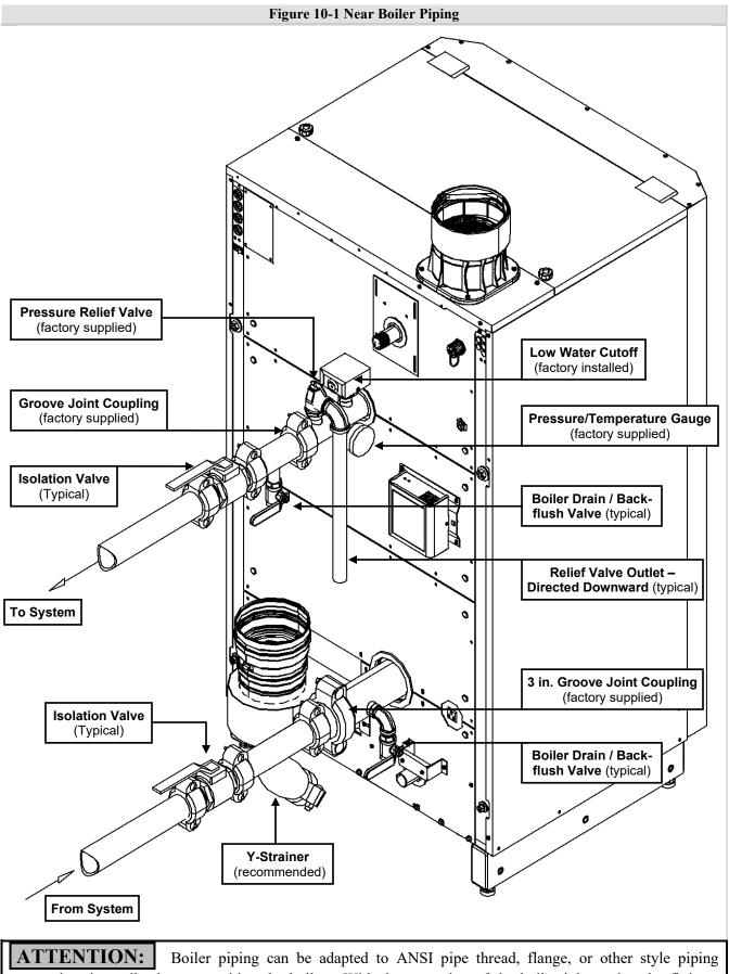
connection, immediately upon exiting the boiler. With the exception of the boiler inlet and outlet fittings, Grooved Joint style piping connections are  $\underline{NOT}$  required.
