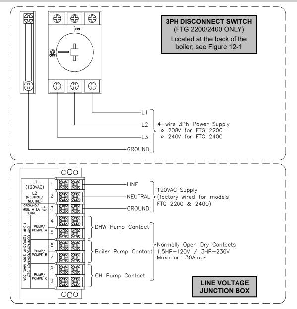
**Fable 12-1** Line Voltage Field Wiring Connections
