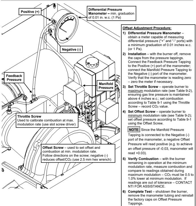
The Gas Valve Offset Pressure is factory set for Natural Gas; units converted to Propane must have the offset pressure field adjusted. Offset pressure must be checked during each annual service for all applications.
