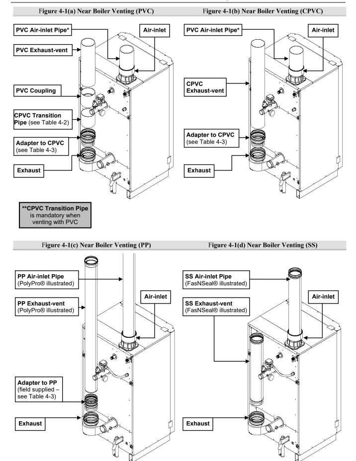
\* Air-inlet - check with applicable local codes for acceptable pipe material.
