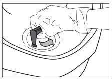
**Step 2**Extract the Cartridge by pulling up on the Key. Tilt the Cartridge in the housing to
