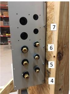
7. Attach enclosure blank side (item #4) to the enclosure using same order as previous step.
