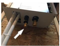
5. Attach the enclosure line set side (item #3) to the back panel and bottom panel.
