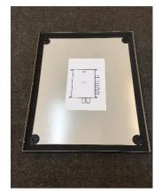
3. Enclosure back (item #1) will mount to structure by piercing rubber grommets. Install two fasteners on right side, back out enough to slide box mounting tabs under fastener and retighten, then install two additional fasteners to the left side.
