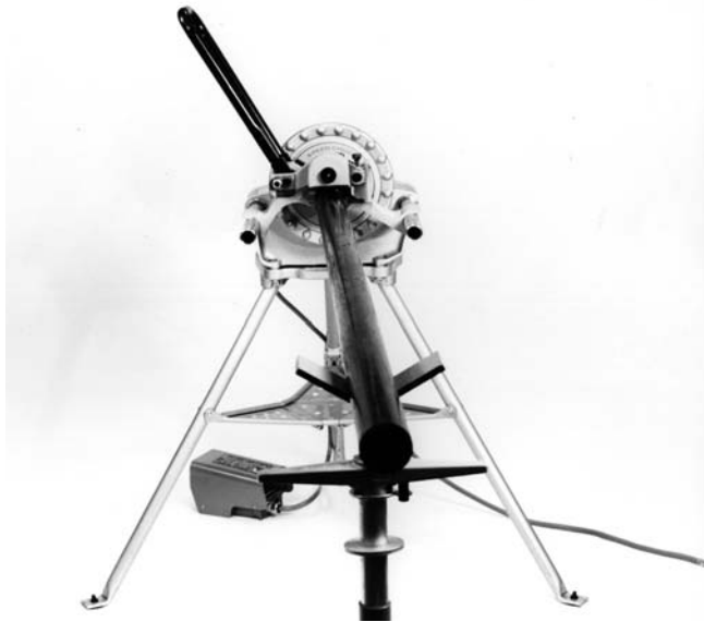
Figure 8B – Operating Machine in FORWARD (FOR) Position
