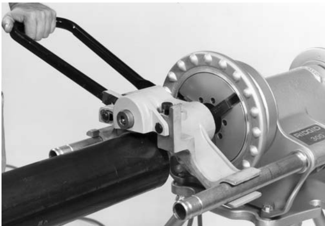
Figure 12 – Forming the Roll Groove
