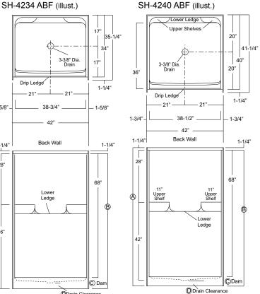
Illustration 1b - Center Drain, Unit Dimension & Alcove Framing Guidelines (dimensional tolerance +/- 1/8")
