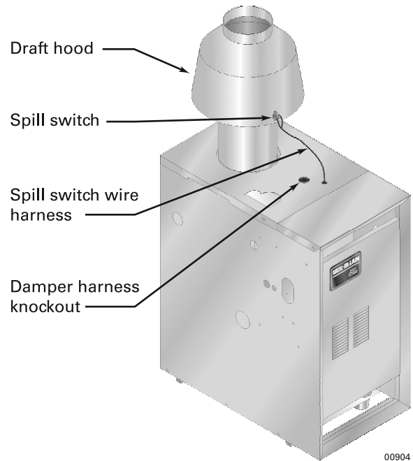
Figure 7 Spill switch with wire harness
