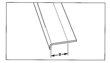
Measure, mark, and cut the left and right vertical panels to window jam depth measurement (B). Trial fit all three panels. If necessary, trim height (C) of the vertical panels to line up with the top edge of the tub or shower wall panels. Sand the cut edges with medium grit sandpaper.
