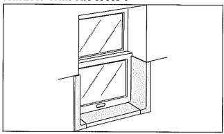
Measure width (A) and depth (B) of the window opening. Cut the sill panel 1-1/2 inches less than the width of the window opening (cut off the end with the factory holes, they are not used).
