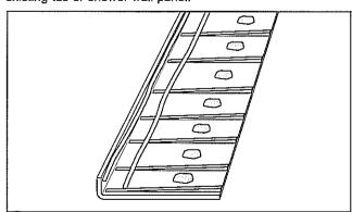
Apply silicone sealant (A) to a vertical panel as shown.
