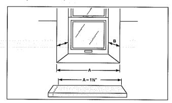
Measure, mark, and cut the sill panel to window sill depth measurement (B). Trial fit the sill panel. Sand the cut edge with medium grit sandpaper.
