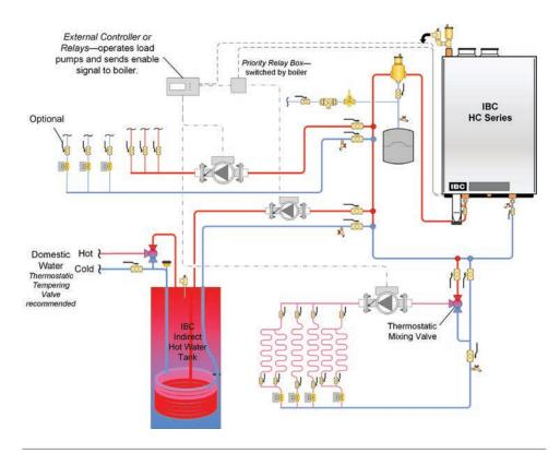
Figure 28: Typical two temperature space heating piping concept with indirect domestic hot water – concept drawing. This drawing is only a simple schematic guide.
