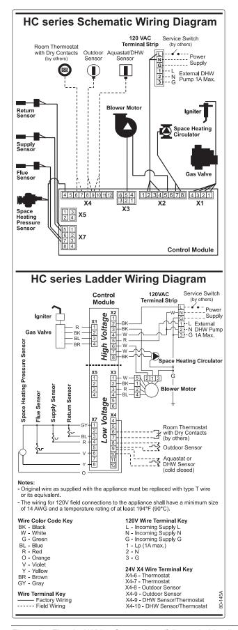
Figure 34: Electrical Wiring Connections (full page ladder diagram at back of this manual)
