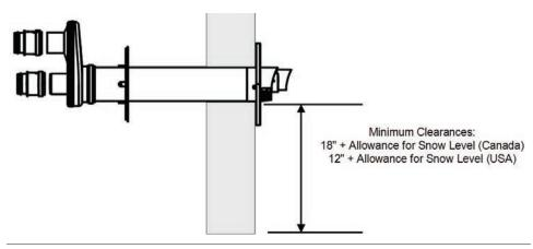
Figure 9b: Horizontal Concentric Termination - Single Kit
