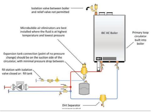
Figure 24: Boiler trim basic options – concept drawing. This drawing is only a simple schematic guide.
