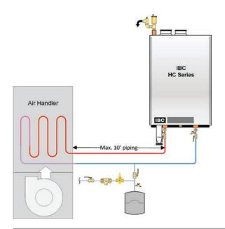
Figure 29a: Air handler and direct domestic hot water – parallel piping concept drawing. This drawing is only a simple schematic guide.
