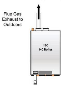
Figure 3: Basic exhaust vent assembly
