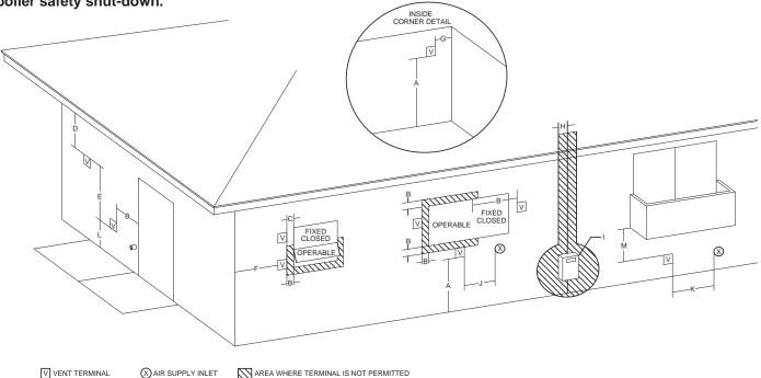
Figure 14: Vent Terminal Clearance
