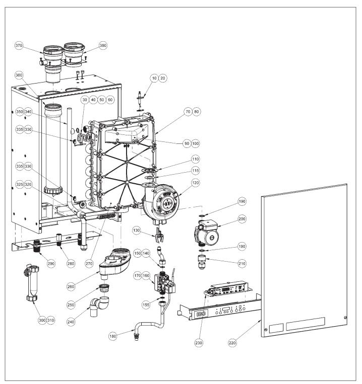
Diagram 6.1-1: Boiler assembly parts
