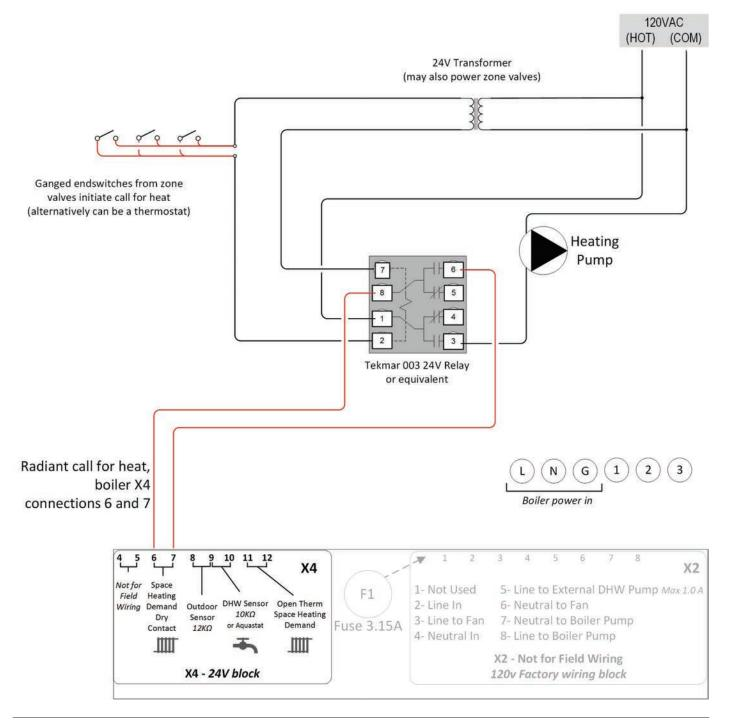
Figure 36: Suggested Field Wiring for Space Heating
