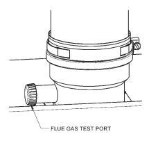
Flue gas test port plug
