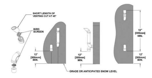
Figure 8: Sidewall vent termination - piping configuration
