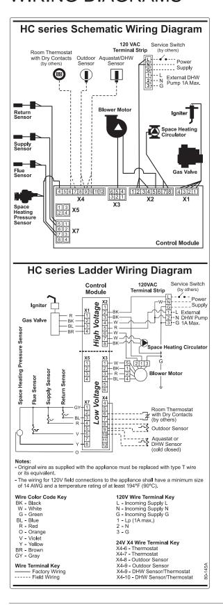
Diagram 6.2-1: Pictorial wiring diagram
