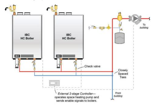
Figure 26: Multiple boiler piping concept – concept drawing. This drawing is only a simple schematic guide.
