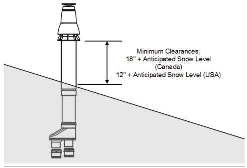
Figure 7: Vertical Concentric Termination - Single Kit
