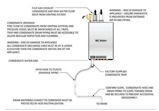
Figure 20: Condensate trap drainage
