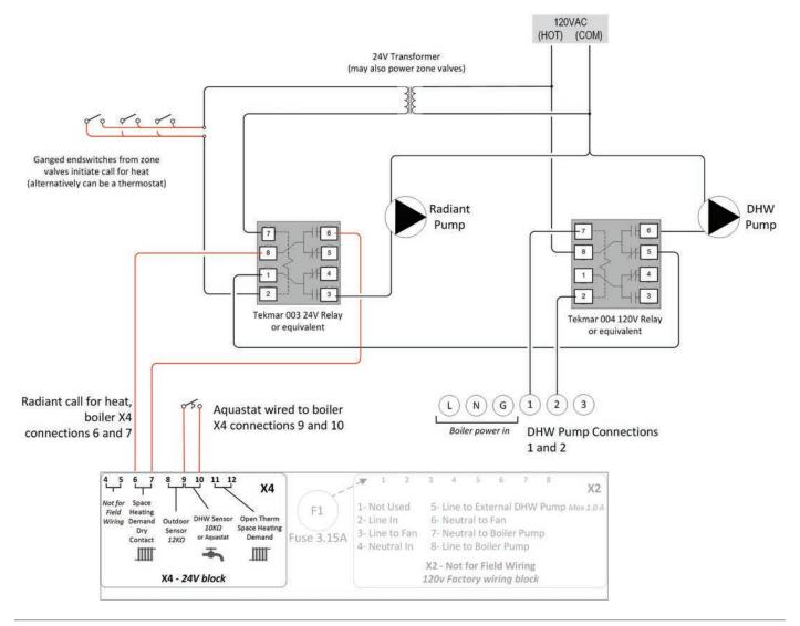
Figure 37: Suggested Field Wiring for Space Heating
