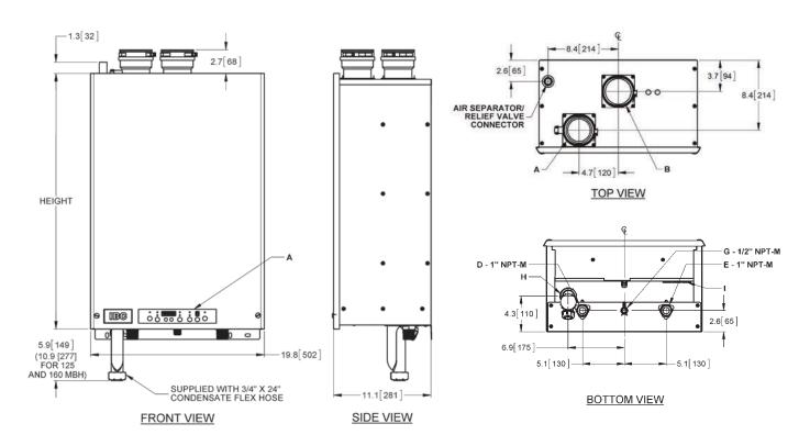
Figure 1a: Dimensions / Connections for HC Series
