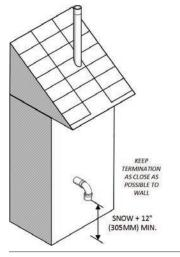
Figure 5a: Rooftop exhaust venting with sidewall combustion air.
