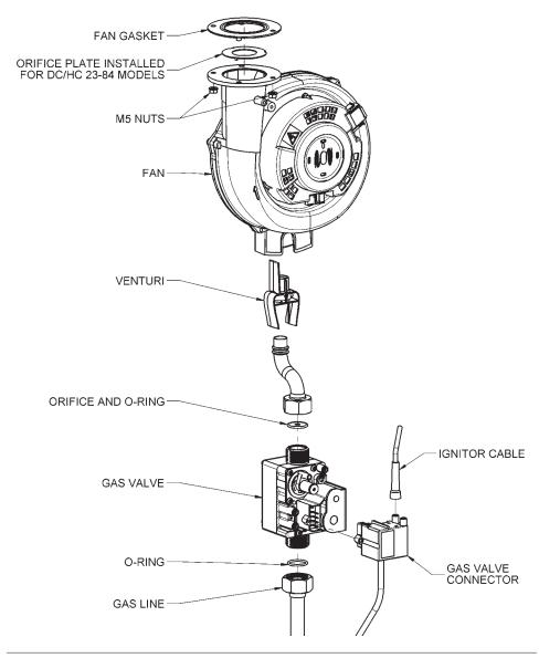
Figure 35: Blower and Gas Valve Assembly
