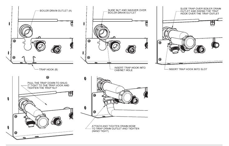
Figure 18: Condensate trap installation
