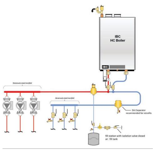
Figure 26a: EZ Manifold Concept Drawing
