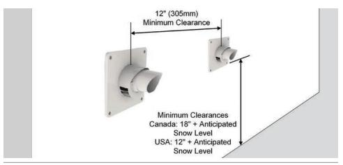
Figure 9a: Horizontal Concentric Termination - Two Kits
