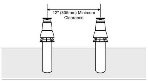
Figure 6: Vertical Concentric Termination - Two Kits
