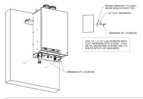
Figure 2: Wall mounting of boiler
