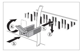
Fig. 56 Securing cables with cable ties
