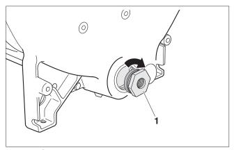
Fig. 24 Sealing the reducer
