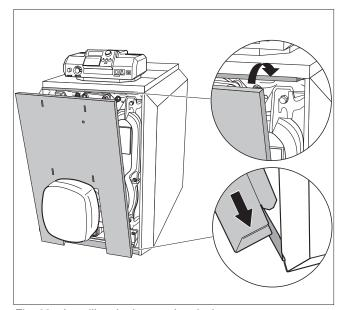
Fig. 63 Installing the burner door jacket
