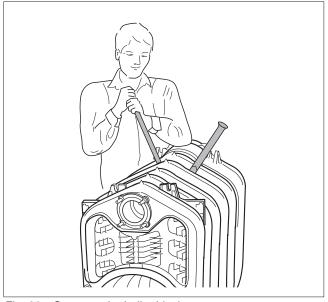
Fig. 26 Separate the boiler block
