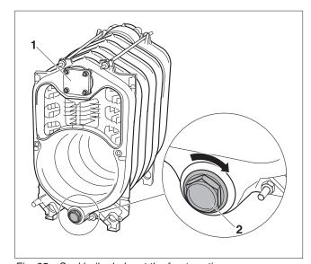
Fig. 25 Seal boiler hubs at the front section
