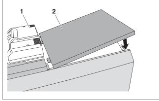
Fig. 57 Install the back boiler cover
