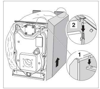
Fig. 40 Slot side panel into place
