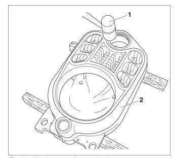
Fig. 10 Knock intermediate section into place
