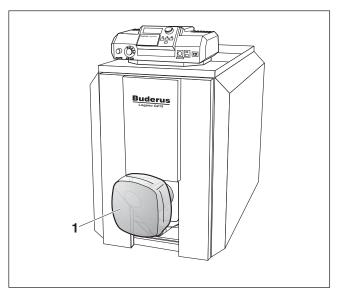
Fig. 71 Resetting the burner
