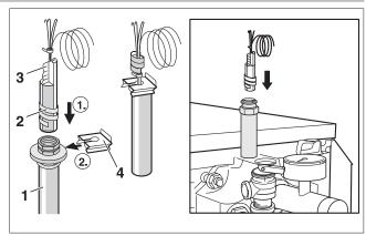
Fig. 55 installing the temperature sensor set
