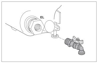
Fig. 48 Installation of boiler drain
