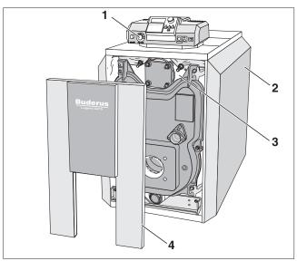
Fig. 1 Boiler without burner
