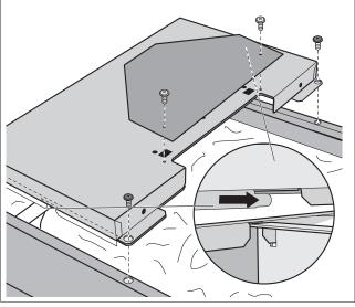
Fig. 42 Installing the front boiler cover
