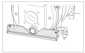
Fig. 36 Fitting the bottom cross bar
