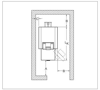
Fig. 3 Boiler room clearances (see Tab. 11)
