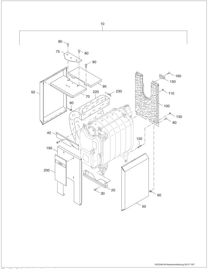
Fig. 77 Boiler block and burner door
