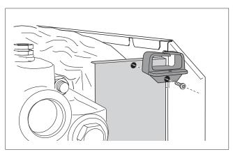
Fig. 43 Fitting the cable entry
