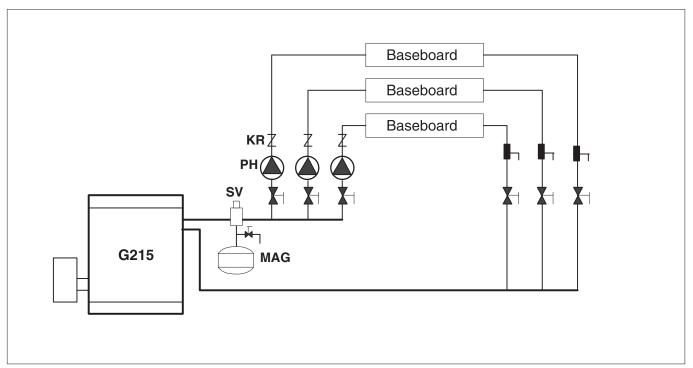
Fig. 73 Multiple circuits with circuit valves
