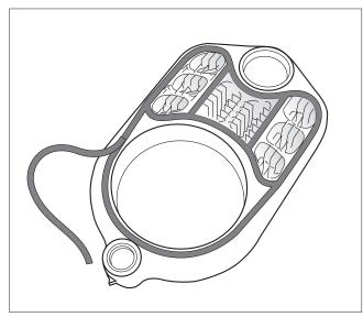
Fig. 9 Inserting the section sealing rope
