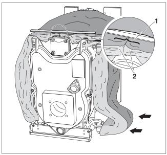
Fig. 37 Installing thermal insulation
