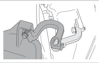
Fig. 32 Hooking on the burner door (here: on the r.h. side) 1  $M12 \times 25$  hexagon bolt
