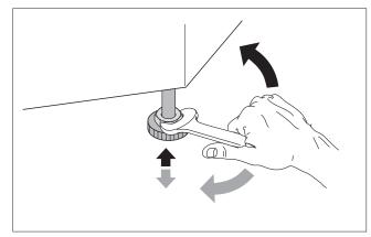
Fig. 44 Leveling the boiler horizontally
