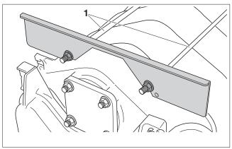
Fig. 35 Fitting the top tie-bar
