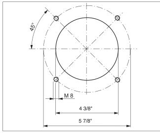
Fig. 51 Burner door mounting holes
