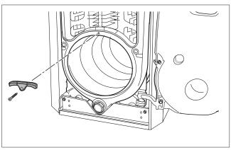
Fig. 62 Removing the blocking plate
