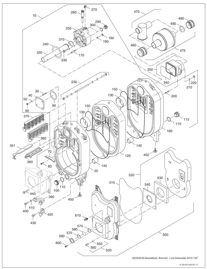
Fig. 76 Boiler block and burner door
