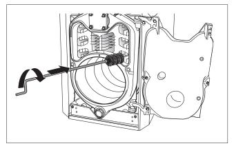
Fig. 68 Brushing out the flue gas passages
