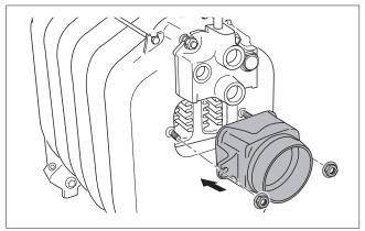
Fig. 23 Fitting the flue outlet
