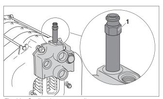
Fig. 22 Sealing the sensor well
