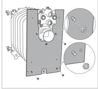
Fig. 34 Installation of the boiler back panel
