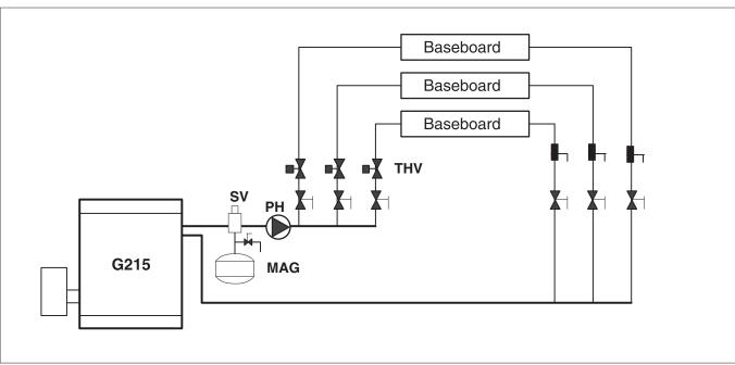
Fig. 72 Multiple circuits with circuit valves
