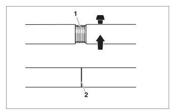
Fig. 12 Making the pull rod threaded connection
