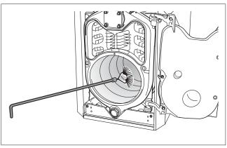
Fig. 69 Brushing out the combustion chamber
