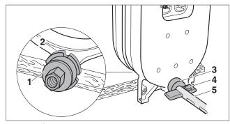
Fig. 14 Compression tool assembled at the lower boiler hub
