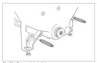
Fig. 33 Spacer pin installation
