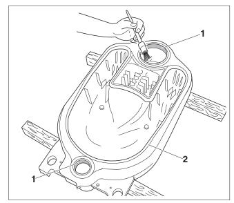
Fig. 6 Coat boiler hubs with red lead putty
