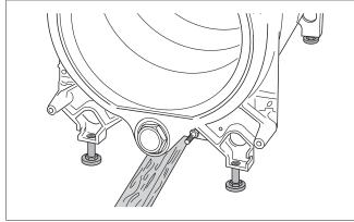
Fig. 28 Fitting adjustable feet
