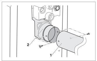
Fig. 45 Installing the flue pipe
