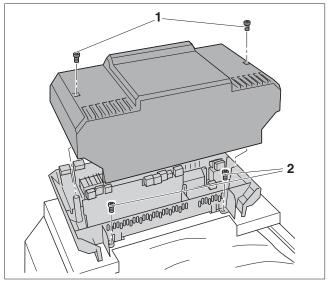
Fig. 53 Removing the cover
