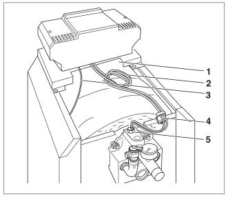
Fig. 54 Routing and connecting cables
