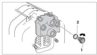
Fig. 21 Seal connections that are not required.
