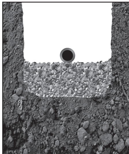
Trench in poor soil
