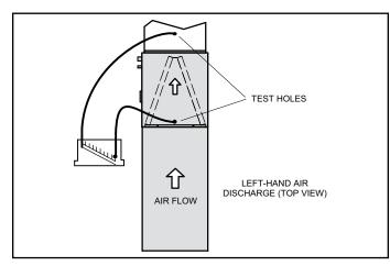
Figure 7. Static Pressure Test
