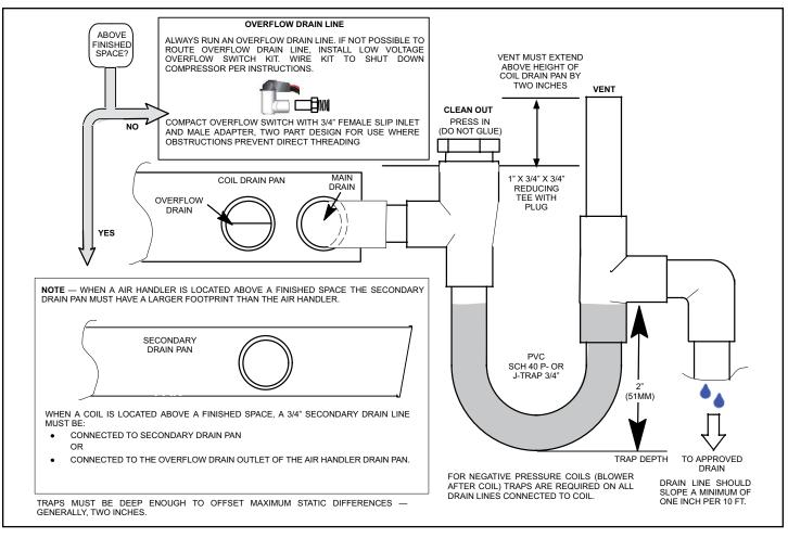
Figure 6. Typical Main and Overflow Drain Installations
