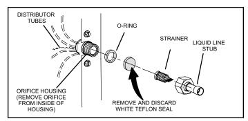
Figure 4. Typical Fixed Orifice Removal
