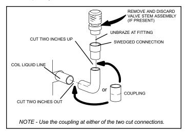
Figure 5. EA\*4X Liquid Line Connections
