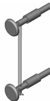
Figure 6.4: Gauge Glass Installation
