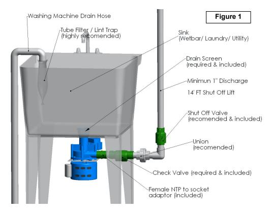
**! NOTE** Sinks will only allow 5-6 gallons-per-minute (GPM) of water to pass through the drain into the pump. When the pump is lifting water to a height of 8 feet, the LTA pump will remove 23 GPM. This causes the pump to turn on and off frequently, or "cycle". The shut off or balancing valve acts to adjust or "balance" the discharge flow to match the inlet flow being let into the pump from the sink, and reduces pump cycling. Adjust pumps as follows to minimize cycling:
