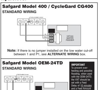
Note: If there is no jumper installed on the low water cut-off between 2 and P1, see ALTERNATE WIRING box.
