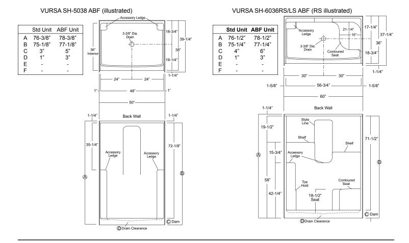
Illustration 1c - Center Drain, Unit Dimension & Alcove Framing Guidelines (dimensional tolerance +0 / -3/8")
