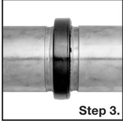
**Step 3.** Install the gasket by placing it over the pipe so that the gasket lip does not extend beyond the end of the pipe. Bring both pipe ends together
