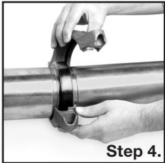
**Step 4.** With one nut and bolt removed, "swing" the coupling housing over the gasket. Verify that the housings are over the gasket and that the housing keys are fully engaged into the grooves.
