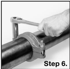
**Step 6.** Tighten nuts uniformly to the recommended bolt torque per Table A. Uneven tightening can cause the gasket to pinch or bind.
