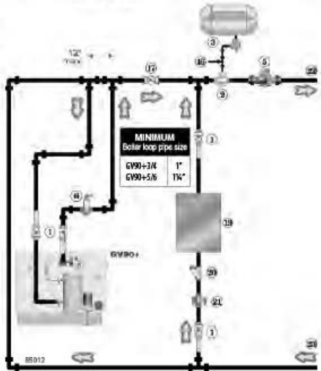
Figure 27 Installing GV90+ boiler in system with water chiller
