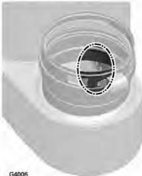
Figure 83 Recuperator flueway drain holes
