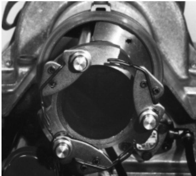
Figure 21 – Machine chucking system set up for let hand operation (e-clips and retainers removed for clarity)
