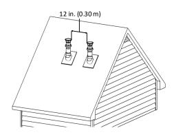
Figure 25: Between terminals at same level
