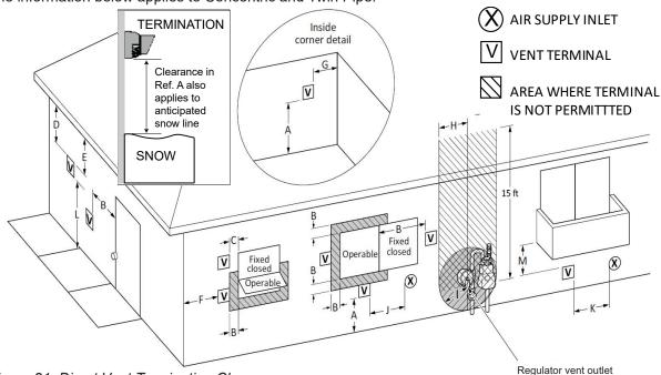
Figure 21: Direct Vent Termination Clearances
