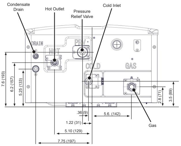
Figure 6: Supply Connections
