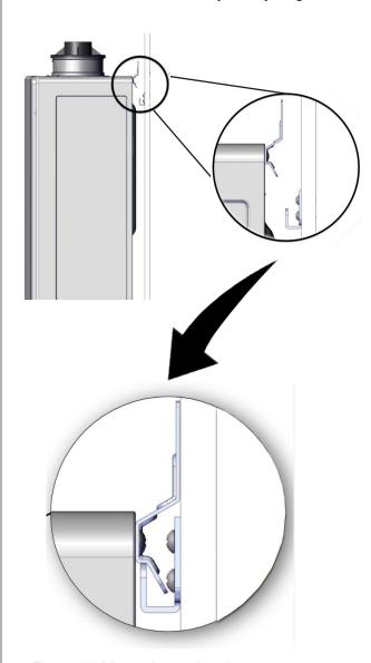
Figure 11: Mount the top bracket
