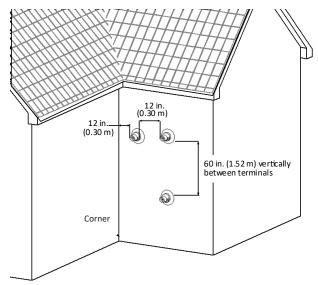
Figure 22: Concentric Pipe Termination Clearances
