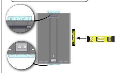
Figure 13: Mount the water heater
