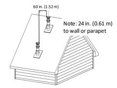
Figure 24: Between terminals at different levels
