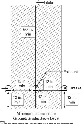
Indicates area in which intake cannot be installed.
