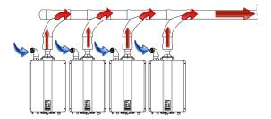
Figure 20: Common Vent, Room Air
