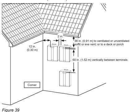
Exhaust Termination Clearances for Internal (Indoor) Room Air Applications
