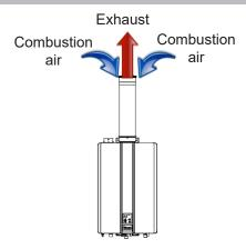
Figure 23: Concentric Pipe
