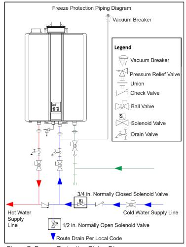
Figure 7: Freeze Protection Piping Diagram
