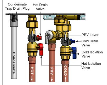
Figure 94: Piping Diagram
