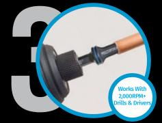
With power tool at MAX speed push bit into the refrigerant line. Keep bit centered & push until the stopper bottoms out, then remove bit from line.
