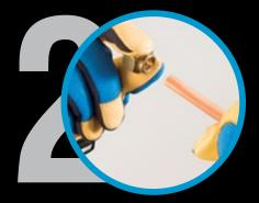
Check the refrigerant line end & ensure it is properly cut & cleaned. Put the flare nut on the refrigerant line & hold the line firmly.
