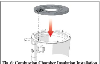
Fig. 6: Combustion Chamber Insulation Installation
