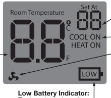
Low Battery Indicator: Replace batteries when indicator is shown.
