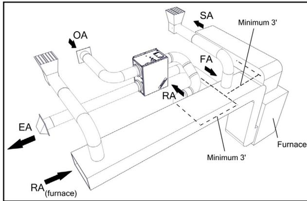
FIGURE 2.4.3 FURNACE RETURN AIR BACK INTO RETURN AIR
