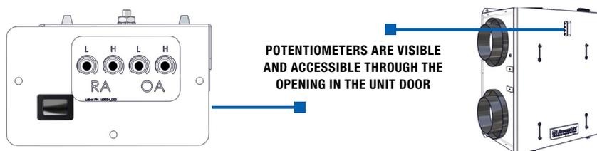
**NOTE:** Adjust low speed fan settings by using the potentiometers marked "L." Adjust high speed fan settings by using the potentiometers marked with "H."
