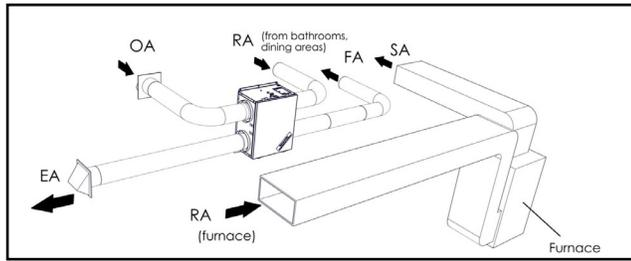
FIGURE 2.4.2 SEPARATE RETURN AIR AND FRESH AIR SUPPLY
