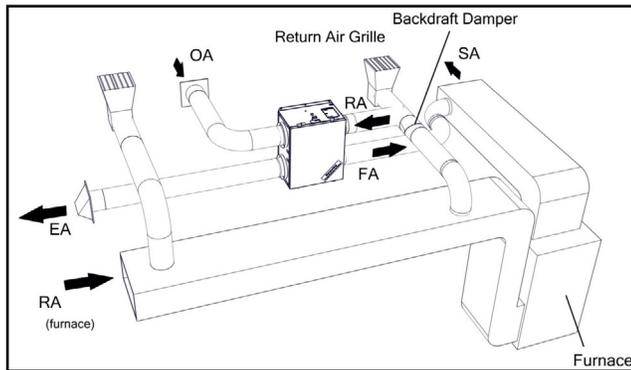
FIGURE 2.4.4 FURNACE RETURN AIR BACK INTO SUPPLY AIR
