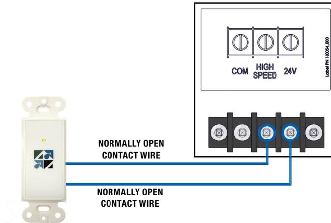
FIGURE 4.8.1 LOW VOLTAGE WIRING DIAGRAM 2
