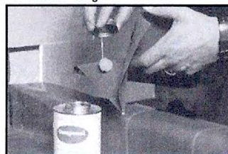
8 Apply Flexible PVC cement to both sides of corner weld
