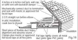
straightest duct routing possible for best performance, and avoid installing the fan with smaller ducts than recommended. Insulation around the ducts can reduce energy loss and inhibit mold growth. Fans installed with existing ducts may not achieve their rated air flow.
