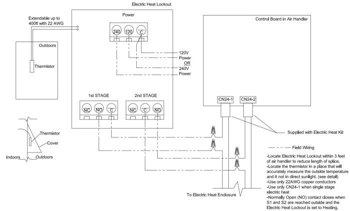
allowing electric heat to energize when called for by the Control Board in Air Handler. -Power for Electric Heat Lockout can be 120V or 240V. See diagram for proper connections
