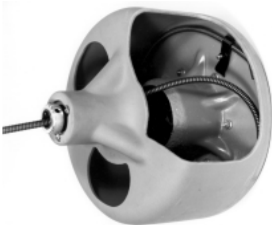
Figure 5 – Coil cable into drum as shown (Drum cut away is for instructional purposes only)
