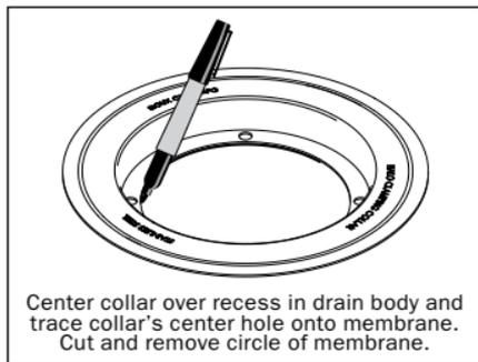
1. Remove drain head and clamping collar and set aside. Lay membrane over drain in the position it will be installed.
